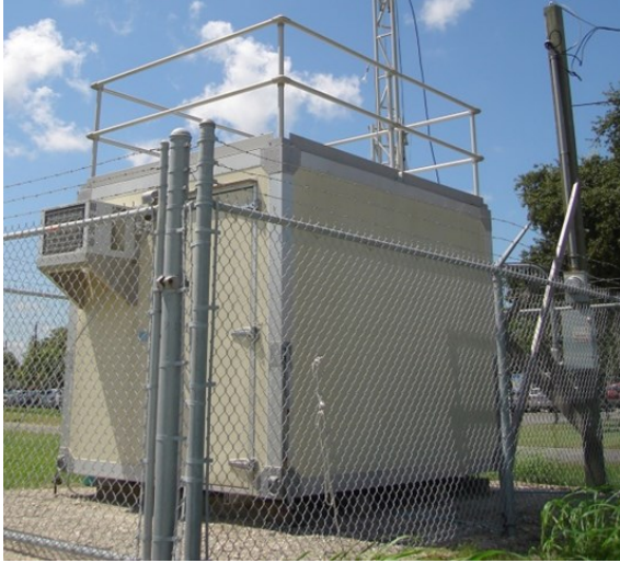
One of the four air monitoring stations installed by the Detroit refinery in 2011. The monitors are operated by a contracted company. The data is sent to the Michigan Department of Environmental Quality.
